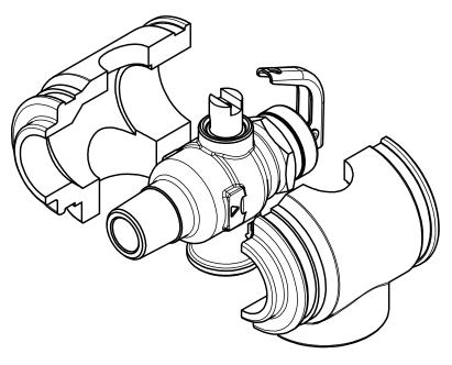
SECURE INSULATION BY WRAPPING THE SUPPLIED ZIP-TIES AROUND THE GROOVES AS INDICATED BY ARROWS
