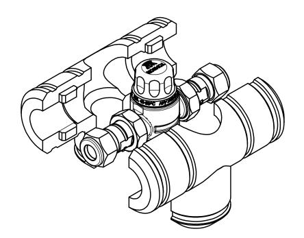
3 SECURE INSULATION BY WRAPPING THE SUPPLIED ZIP-TIES AROUND THE GROOVES AS INDICATED BY ARROWS
