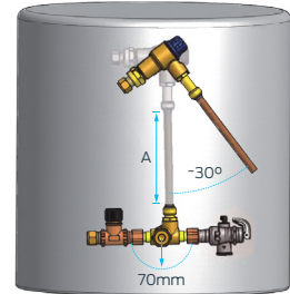
Diagram 2 – Installing Cold Supply From Manifold to Tempering Valve
