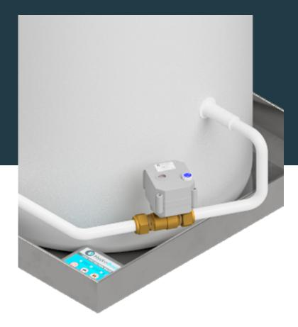
The HydroBoss Leak Protection Valve is an electronic automated shut off valve for use with a mains water supplied water heater installed with a safe tray that is not plumbed to waste. In the even of a leak, accumulated water in the safe tray is detected by the valve sensor and the water supply is isolated. The valve is designed to be installed in the water supply pipework, adjacent to the cold water inlet of the water heater and upstream of any expansion control valve (if fitted).
