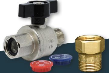
The RMC FloodGuard range has been designed to reduce the extent of flooding and water damage caused from burst flexible connection hoses. In the event of excessive water flow or hose burst, the valve automatically snaps shut to minimise water escape and damage.
